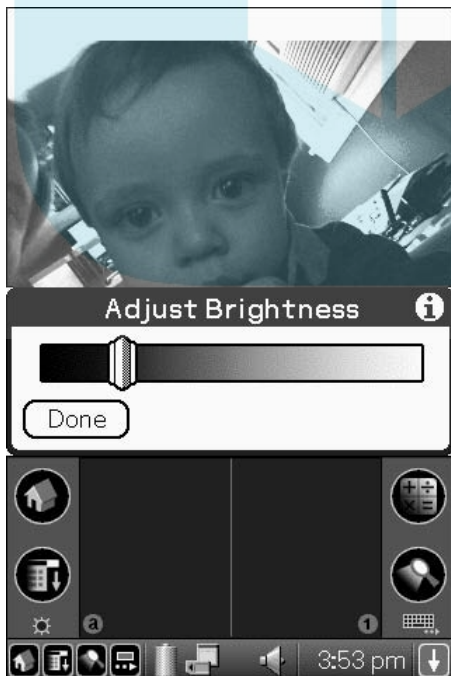
Figure 20-3: Turning the brightness level down to the lowest comfortable level can greatly improve battery life.
